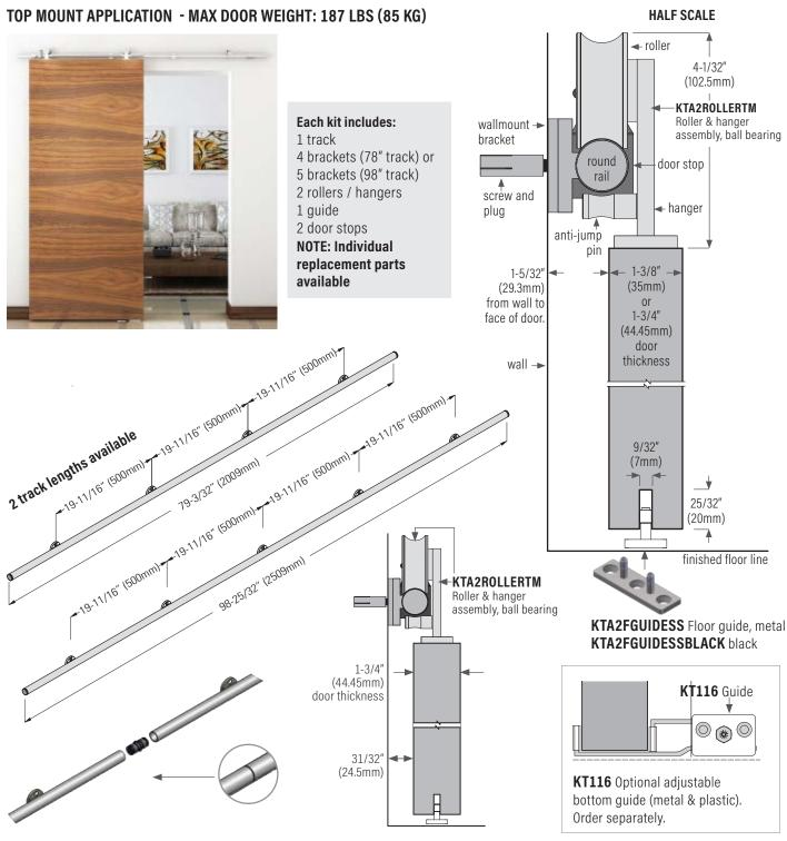
KTA2RAILCON Connector piece, connects 2 pieces of rail end to end. Order separately.
