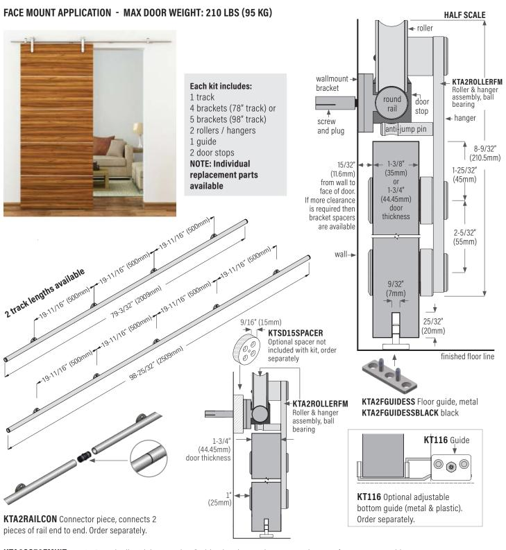
KTA2SS78FMKIT A2 Round rail, stainless steel, 78" with 4 brackets, 2 door stops, 2 hangers face mount, 1 guide
