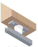
mounting plate surface mounted on bottom of door
