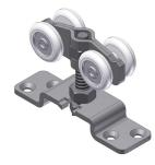
**KT40PDKIT for 1 door application:** (Hardware kit **not included** with frame, order separately) KT40HANGER (2 ea) hangers, KT107 (1 ea) jamb mounted guide, KT155 (1 ea) wrench, installation sheet plus all screws.
