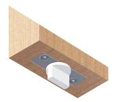
mounting plate mortised into bottom of door
