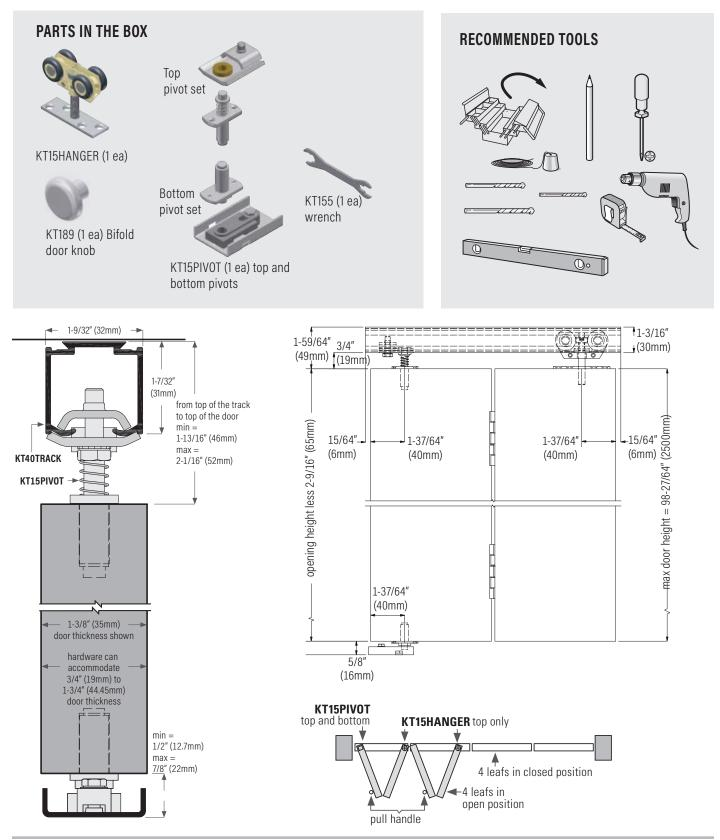
Fit top and bottom pivots into holes and screw in long wood screws. Fit hanger with door plate surface mounted. Hinge doors together with 3 hinges per joint as shown below. Doors over 2100mm high will require 4 hinges per joint.
