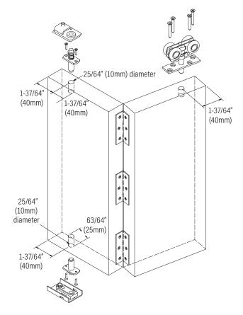
Doors over 17-23/32" (450mm) wide or with weight in excess of 15kg need stabilizing with KT120 door guide fitted plumb under top hanger(s) and engaging KT20 floor channel. Minimum door thickness must be 1-3/16" (30mm). Not included in standard kits.
